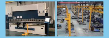
Fabrication job seems easy, but high quality fabricated pump packages can never be as easy as thought. We invested huge money to import high precision assembling tables from Europe and they are playing a very important role in our copping and assembling process for manufacturing pump skids, fuel tanks and canopies.
